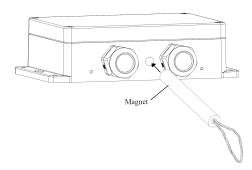
A short touch (< 2 s) enables the automatic mode, a touch of 2...10 s — manual mode. The activation of the automatic mode is followed by a single LED blinking and acoustic signal. If manual mode is activated, the double acoustic and light signal follows.
